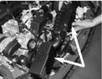
9- Loosen the 2 screws holding in the MAF sensor using the Philips screwdriver and remove the MAF sensor from the
