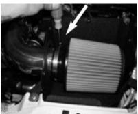
23- Position for the best fit, secure and tighten the clamp.
