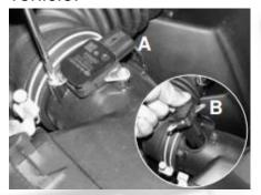
10- Install the MAF sensor into the intake pipe.
