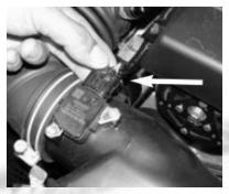
6- Un-clip the upper part of the air box, remove the upper assembly including the intake tube from the vehicle.
