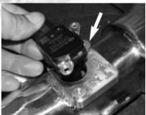
11- Secure MAF sensor using provided button bolts.
