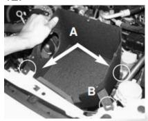
15- Secure the front of the heat shield using provided bolt and washer.
