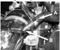
25- Cap off the sound tube resonator with provided vinyl plug.
