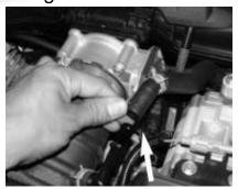
3- Loosen the clamp on the Sound Tube resonator.
