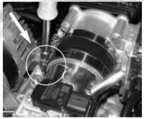
24- Secure the crank case line to fitting on pipe using pliers and factory clamp. Reconnect the MAF sensor harness.
