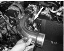
22- Install the filter to the intake pipe and tighten the clamp.
