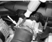
2- With pliers, pull back the crank case line from the intake fitting.
