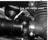
5- Disconnect MAF sensor harness and pull line away from air box.
