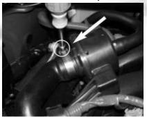
4- Loosen the clamp on the intake tube and remove the sound tube. This will no longer be used on the new intake system.
