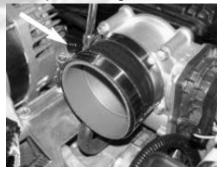
20- Install the intake pipe through heat shield and position to throttle body.
