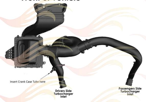
Remove the 2 plastic retaining rivets from the air scoop and remove scoop from engine bay.
