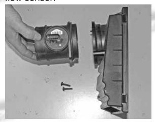
17- Remove the "O" ring from the mass air sensor.
