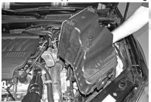
8- Remove the transmission control module from the housing, release the clamshell retaining clip, and then disconnect the wiring harness.
