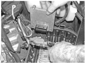
9- Release the engine control module from the mounting clup and lift the module from the base.
