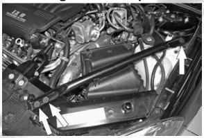
6- Depress the 4 air box housing retaining clips.
