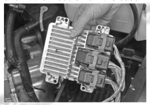
10- Release the engine control module wiring harness clamshell clips and disconnect the wiring harness from the engine
