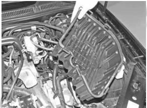
12- Remove the 2 mounting grommets from the inner fender, and then reconnect the engine control module wiring harness. Use the provided zip tie to tie them in the inner fender.
