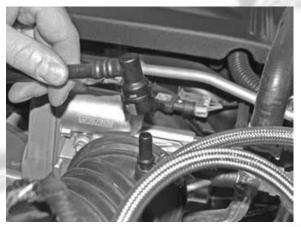
3- Loosen the hose clamp, which secures the intake tube to the throttle body, and release the air box over center clips.
