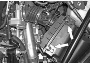
4- Remove the air box housing half and stock intake tube.
