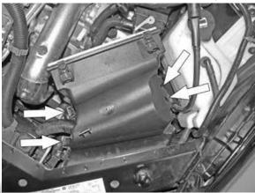
7- Remove the upper air box housing from the vehicle.
