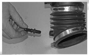
15- Lossen the hose clamp, which secures the stock intake tube to the mass air flow sensor, and then remove the hose from the sensor.
