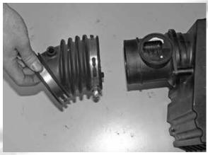
16- Remove the 2 screws, which secure the mass air flow sensor to the air filter housing and thenremove the mass air
