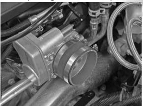
14- Remove the crank case vent fitting from the stock intake tube.
