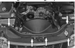
10- Remove the six grill retaining clips from the grill, then tilt the grill forward and lift to remove from the vehicle.
