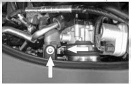
4- Pull the intake plenum off the throttle body and rotate forward, then disconnect the crank case vent hose from the tube attached to the intake plenum. **NOTE: Do not**
