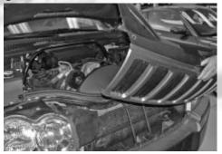
11- For 6.1L engine, remove the upper fan shround is necessary.
