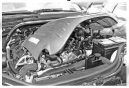
7- Remove the crank case vent hose from the engine.
