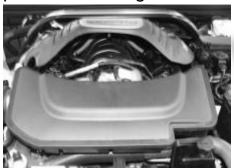
3- Remove the intake plenum-mounting bolt and loosen the intake plenum hose clamp at the throttle body.
