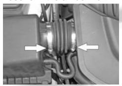
2- Remove the oil filler cap and then lift up the front of engine cover to gain access to the throttle body hose clamp intake plenum mounting bolt.
