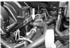
8- Un hook the air box lid retaining clamps and then remove air box lid and filter.
