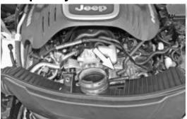
5- Disconnect the air temperature sensor electrical connection and then remove the intake plenum from the vehicle.
