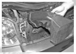
13- Remove the air box mounting bolt.
