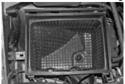
14- Lift the lower air box and remove it from the vehicle.
