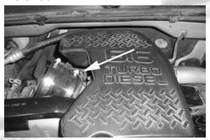
11- Loosen the bolt as the arrow point so the tab on the heat shield can sandwich between the washer and the grommet.
