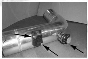
8- Assembly the 2 pieces heat shield with provided 4 washiers, bolts, and nuts.
