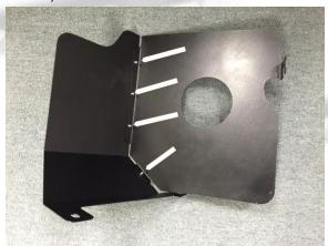
9- Install the provided rubber trim around the edges of the assemblied heat shield. Place the velocity stack adapter in the heat shield and install the supplied elbow coupler making sure the coupler is pushed completely against the heat shield. Once the adapter and coupler are tight against the heat shield, snug the clamp to hold it in place but do not
