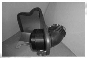
10- Install the reducer coupler with 2 clamps onto the turbo and securely fasten. Also make sure the intake pipe clamp is installed but left loose enough until the intake pipe is installed.
