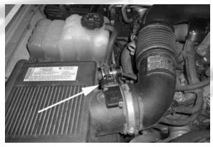
2- Loosen the clamp at the turbo.
