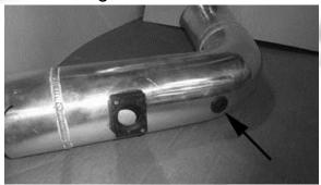
7- Install the MAFS and the air filter reminder into the intake tube.
