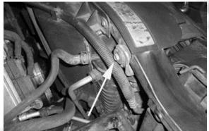
12- Install the heat shield into the vehicle by reusing 2 of the bolts removed from step 4. Also make sure the tab is placed between the washer and grommet that was loosened in step
