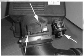
6- Install the grommet in the intake.
