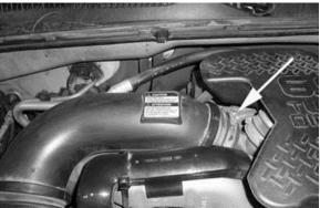
3- Lift the stock intake tube and air box assembly up and out of the vehicle by pulling up and out firmly.
