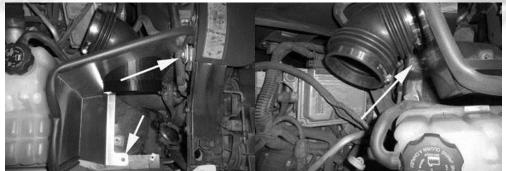
13- Install the intake pipe into the vehicle, position it and once pipe is in desired location tighten the clamps.
