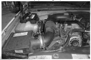
4- Remove the 5 bolts and remove the stock air box tray from the vehicle.
