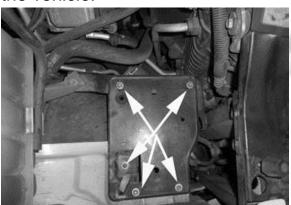
5- Remove the Mass Air Flow sensor and the air filter reminder.
